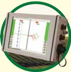
Vehicular PC with 8.4" touch screen display and integrated GPS RTK receiver. This solution reduces to a minimum wiring and makes easier to move it in different tractors.
