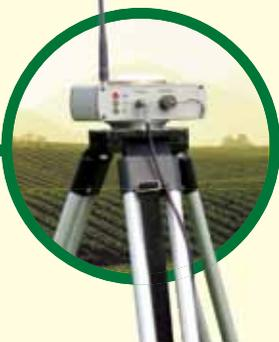
RTK GPS base station with integrated radio modem and GPS antenna.
