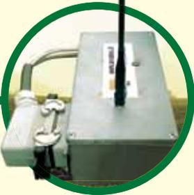
Controlbox to control cross alignment with dual axis inclinometers, radio modem, installation kit to perform the automatic positioning of every single plant without wire (optional).
