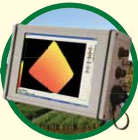
Board computer with 8,4" touchscreen display and integrated GPS RTK rover. This solution: reduces wiring, makes it easier to move it to different tractors and allows to graphically display earthworks.
