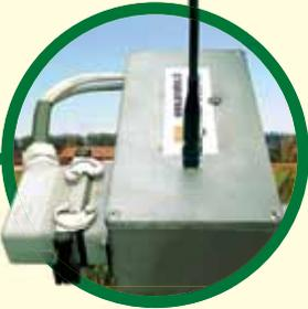
Control box to control the blade vertical displacement with integrated radio modem. The unit has a small size (25x15x10 cm)
